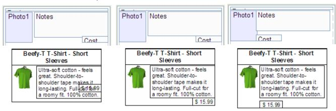
In the first example in this group, we've allowed the Cost Field to overlap the Notes Field. When two fields overlap vertically, the separation rule between them is cancelled. The Notes Field still grows but does not affect the Cost Field and now the separation between the Product and Cost Fields can be seen. The Cost Field appears to move up slightly but is in exactly the same place it would be if there were no data in the Notes field.
